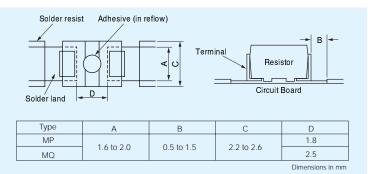
When parts are mounted on a board in high density, solder can possibly attach to the resistors in an excessive amount to affect performance or reliability of the resistors. To prevent this effect, the use of solder resist is recommended to isolate solder lands.
